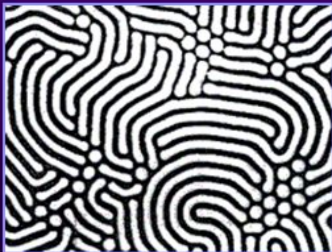
Ferromagnetic garnet film Period \sim 10^{-5} m
