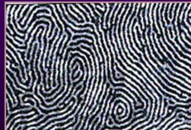
Block copolymers Period \sim 4 \times 10^{-8} m
