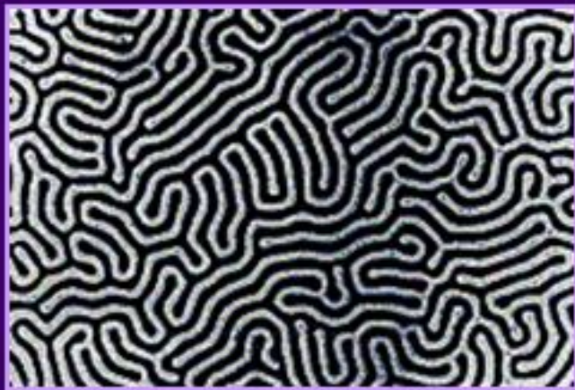
Ferrofluid confined between two glass plates Period \sim 1 cm
