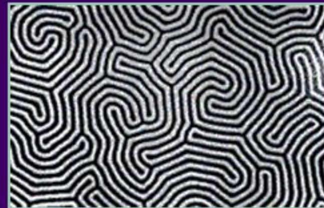
Ferromagnetic garnet film Faraday effect Period \sim 10^{-5} m
