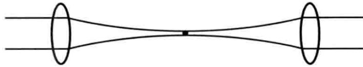
Fig. 11.1 Schematic illustration of a dipole potential. A laser beam incident from the left is focused by a pair of lenses. A typical intensity profile is given by Eq. (11.12) which produces a harmonic potential near the center (indicated by the dot), where atoms are trapped.
