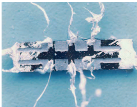
Figure 28: The sample used to discover the fractional quantum Hall effect. Courtesy of Ady Stern.
